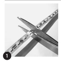
Handle strip with care. Cut with sharp scissors or snips on the dotted lines only.
