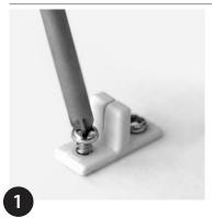
Fix clips with 1 suitable screws (min. 5 clips per metre or every 250mm/9.84").
