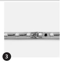
Press in position, avoiding direct pressure on LEDs.
