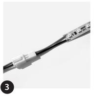
Check polarity and test prior to mounting (see also relevant Wiring Guide).
